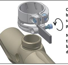
Open the feedneck by tightening the screw against the plastic shim.
