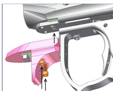
The foregrip extender is designed to be a close, tight fit between the transfer plate, frame, and extender. Manufacturing differences from marker to marker require that a small gap be present, however this will not affect regular gameplay. Excessive playing in mud, rain, swamps, or other wet conditions may require you to clean the sensor board if any foreign liquid is able to seep inside the marker (however this is normal wet playing conditions).
