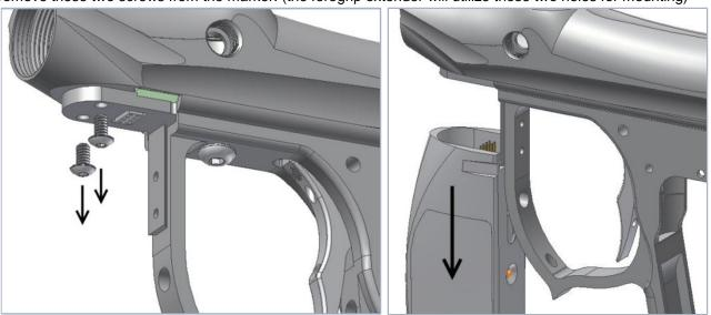
3. Loosen the two screws holding the marker's frame to the body. You will need to create a small gap between the frame and body in order to proceed with the installation (you can remove the frame entirely if you wish). Warning, the firing assembly may become free when the rear frame screw is loosened.
