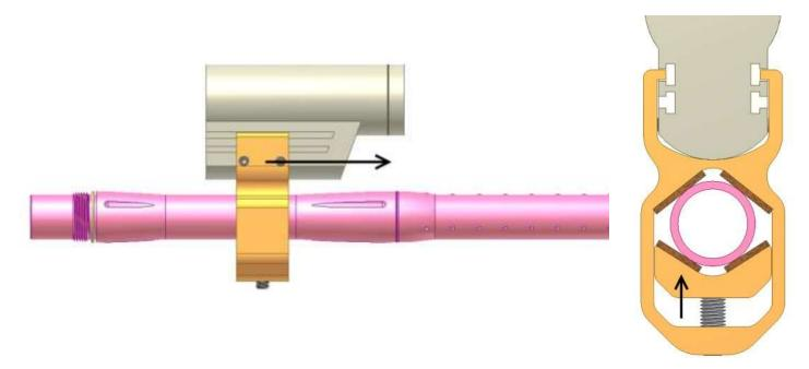
Note: if using a two-piece barrel system, the camera mount is compatible with either section of barrel. Installing it on the barrel back will balance the marker better, however installing it on the front may give you a better vantage point for videos.
