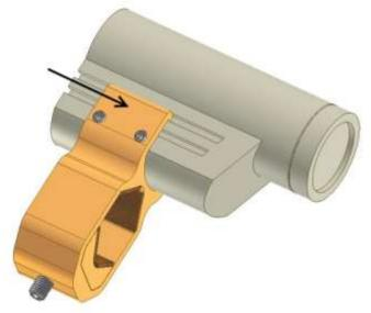
3. Gently tighten down the small set screws to lock the camera in position. For best results, tighten each of the four screws to "suspend" the camera within the mount.
